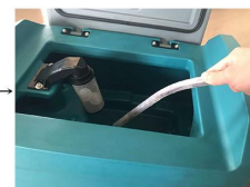
9.Finish the work rinse the sewage tank with clean water
