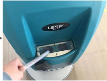
5.Remove the bush plate rise and fall pedal and put down the brush disk cover
