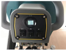
6.Turn on the brush plate motor switch and the suction rake motor switch
