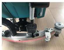
5.Remove the bush plate rise and fall pedal and put down the brush disk cover
