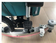
5.Remove the brush plate rise and fall pedal and put down the brush disk cover
