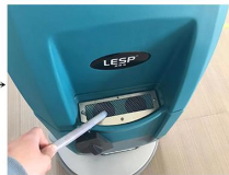
5.Remove the brush plate rise and fall pedal and put down the brush disk cover
